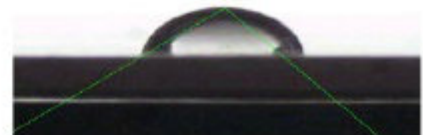
Sessile drop measuring static contact angle
