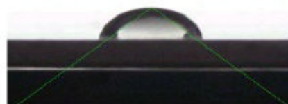
Sessile drop measuring static contact angle
