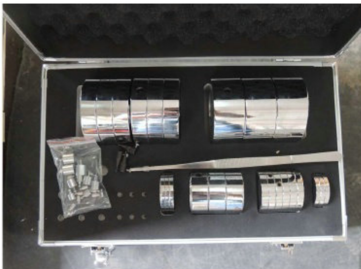
Accessories containing case: (Weights, needle indenter, pressing head, tweezers etc.,)
