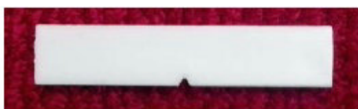
Plastic V notch impact sample 80*10*4mm
