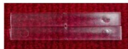
Organic glass V notch impact sample 80*10*4mm
